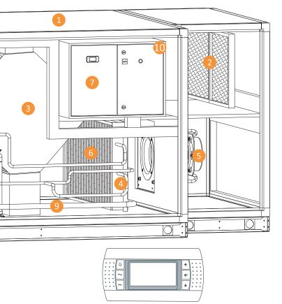
The thermal capacity delivered by the heat pump unit will be continuously modulated through the speed variation of the DC brushless rotary or scroll refrigeration compressor.
